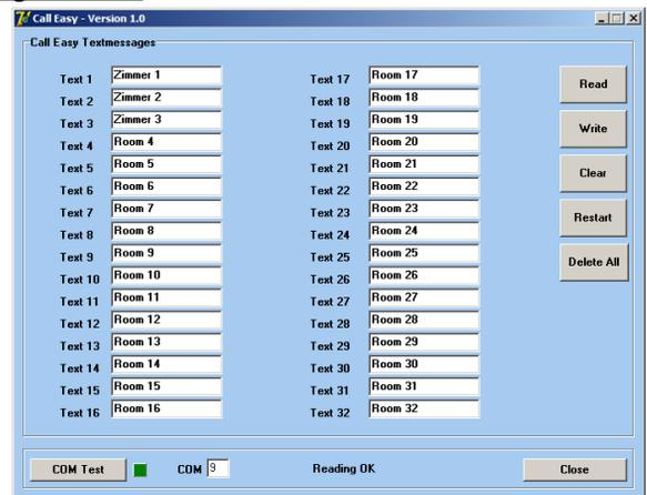
Connect the Call Easy with your computer and change into programming mode with the programming switch on the rear side using the paper clip. Run the program, set the right COM port where Call is Easy is connected and click on „Connect“
